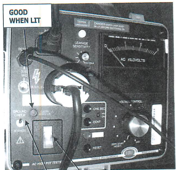
GROUND CHECK & OFF/ON ROCKER SWITCH
