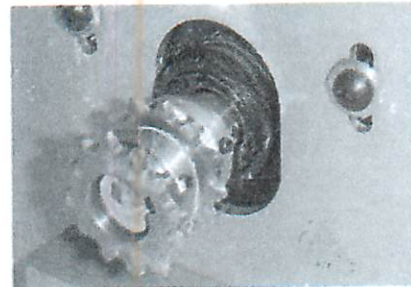
(2) DRIVE SPROCKETS HUB INWARD ON MOTOR SHAFT, 8-32 X 1/4 SS ON KEY
