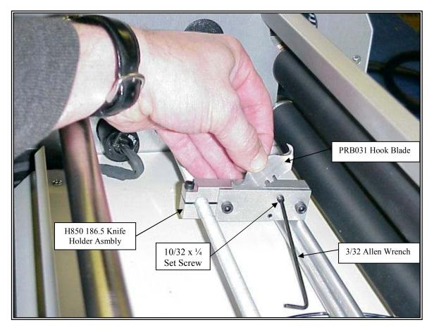
Secure hook blade in knife holder assembly, with allen wrench, in position depicted below
